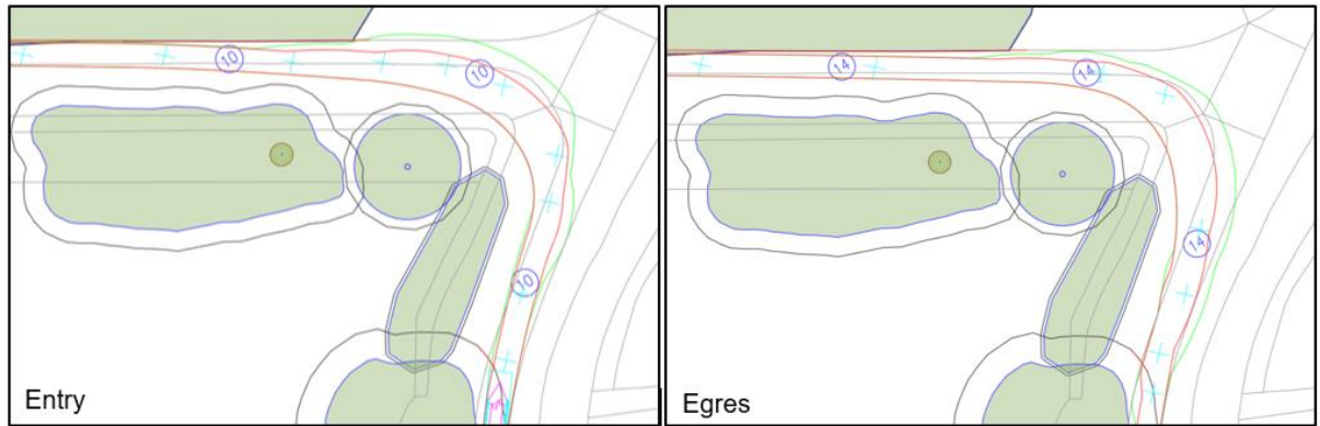
Figure 43: 1000T Crane Swept Path Analysis Entry and Egress: Weirs Drove/Newnham Drove Junction
